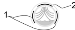
FIGURE 3. SOS™ SENSOR WITH THREE ROUNDED PLATES. ELECTRODE #1 (2 PLATES) AND ELECTRODE #2 FUNCTION AS THE CAPACITOR PLATES, AND THE WATER IN THE DRAIN PIPE AS THE DIELECTRIC.
