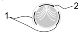
FIGURE 4. SOS™ SENSOR IS ACTIVATED WHEN THE DRAIN PIPE IS COMPLETELY FULL OF WATER.
